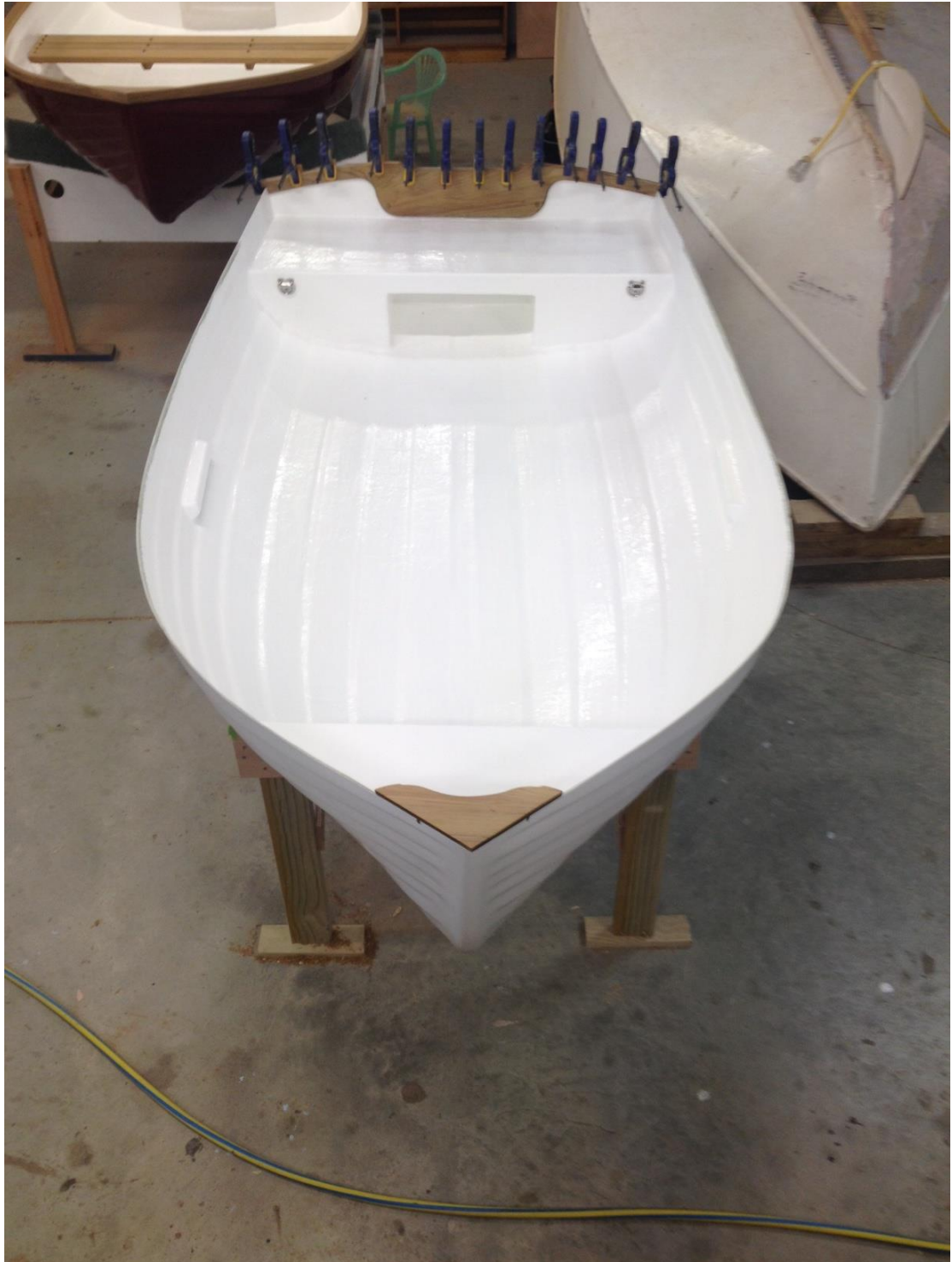
Bow plate installed using West System epoxy and marine grade 316 stainless steel fasteners.
