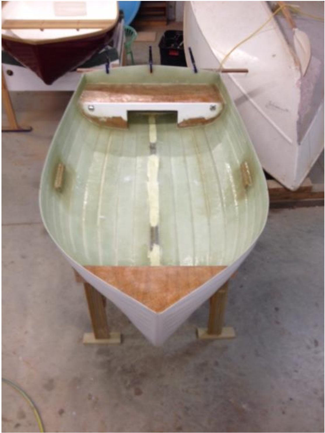
The tank seats are installed.
