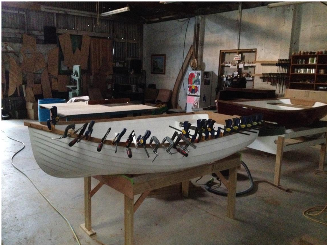
Gunnels glued on using epoxy and a few clamps.
